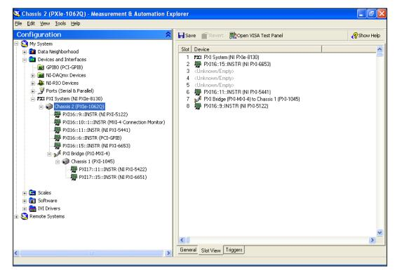
Figure 2-5. Multichassis Configuration in MAX
